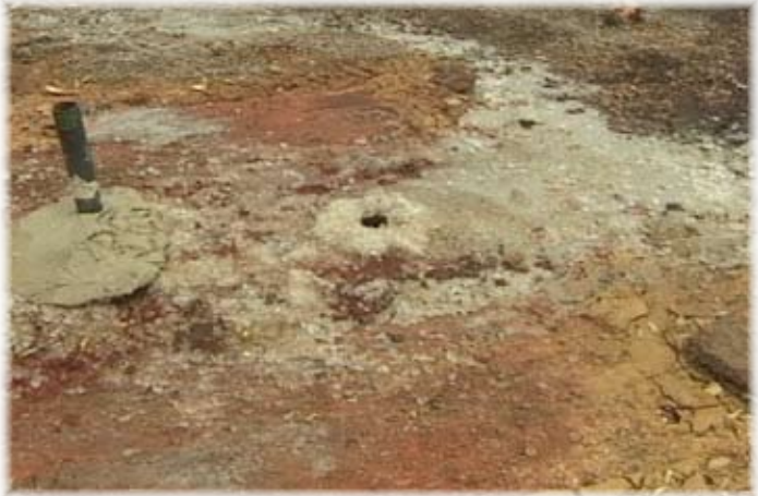
An unprotected drilling hole from which groundwater is leaking
